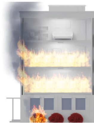
90 minutes: Fire contained within cavity compartments 1 and 2
