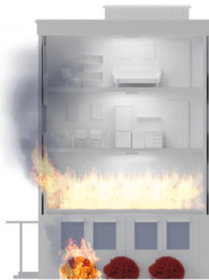
60 minutes: Fire contained within cavity compartment 1
