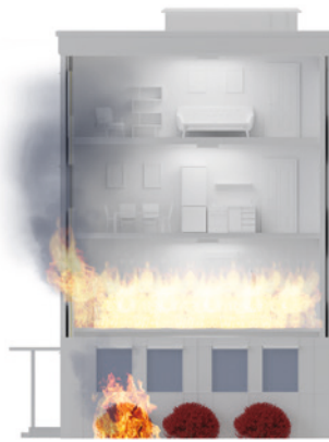
60 minutes: Fire contained within cavity compartment 1
