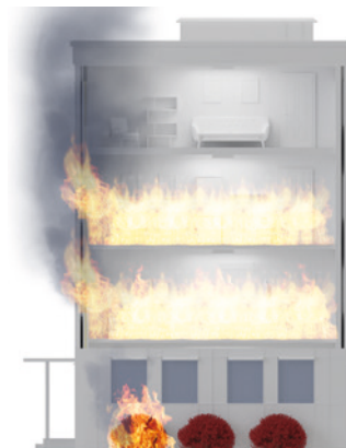
90 minutes: Fire contained within cavity compartments 1 and 2
